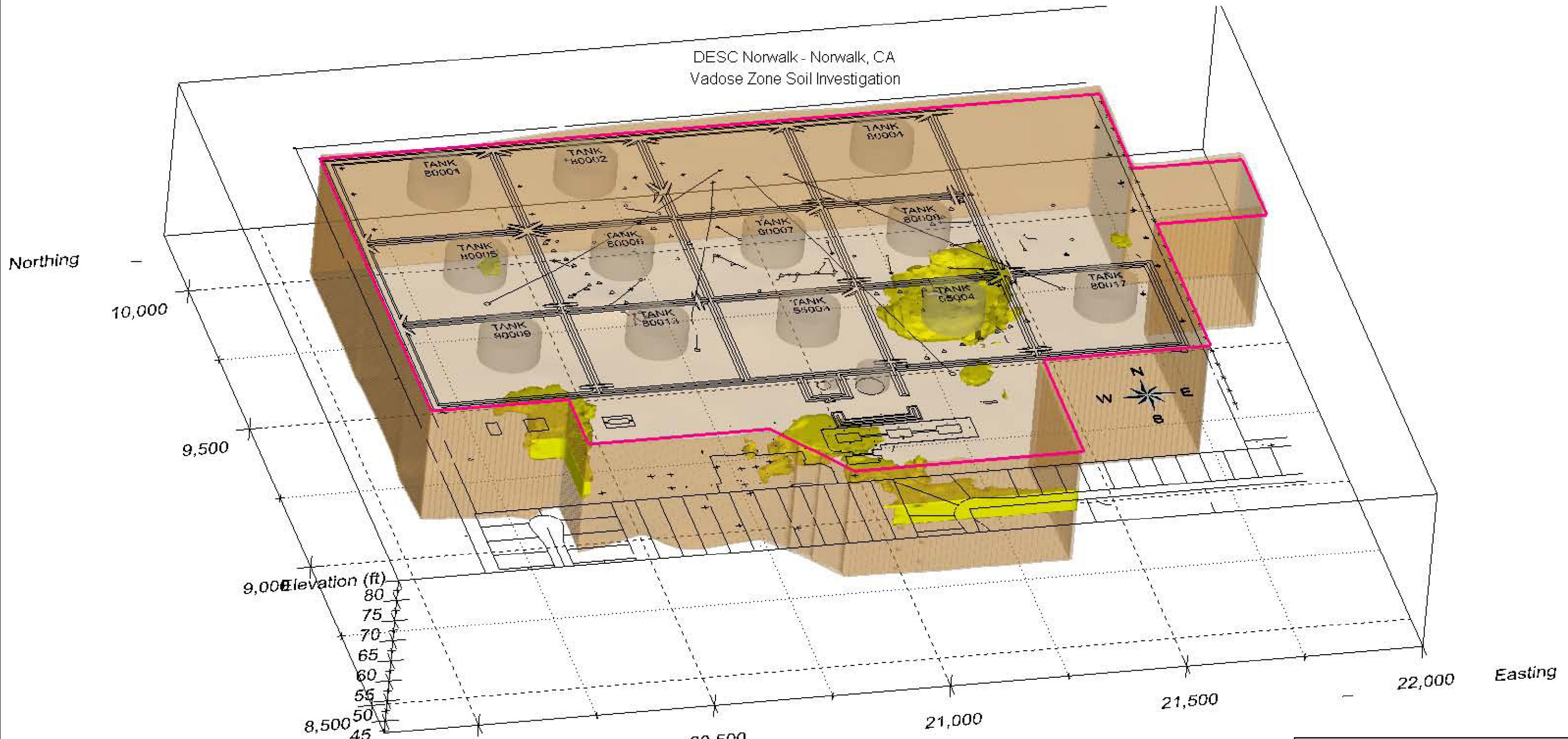
FIGURE B-5 IMPACTED SOIL FROM 10 TO 15 FEET BELOW GROUND SURFACE DEFENSE FUEL SUPPORT POINT NORWALK, CALIFORNIA PARSONS Pasadena, California
